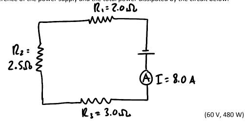
17) Find the value of  $I_1$  and the total power used by the circuit. **25.0**
