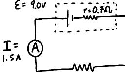
5) What is the terminal voltage of the <u>battery in the circuit shown</u>?
