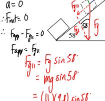
A 15 kg block sits on an inclined ramp whose coefficient of friction is 0.21. Find the block's/acceleration.
