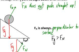
For inclined plane questions our first step should always be to resolve the object's Fg into two companents:
